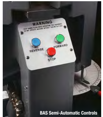
BAS Semi-Automatic Controls
