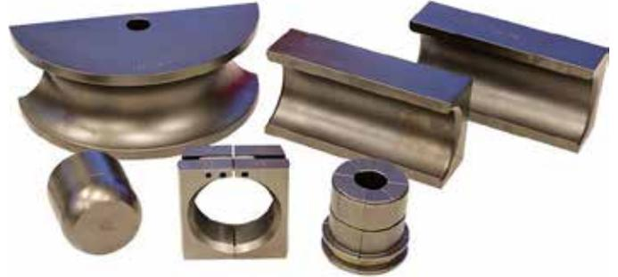
All BendPak tooling is precision-machined from solid steel. After the CNC machining process, the tooling is gas-carburized, oil-quenched and heat-treated to a minimum hardness of 58 Rockwell. No cast or ductile (brittle) iron is used in the manufacturing of any of our tooling.
