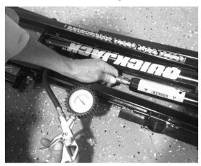
3. When the pressure is between 40 and 50 PSI / 2.75 to 3.4 BAR, remove the pump or air compressor.
