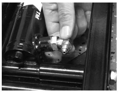
3. Position the threaded fitting end as shown above; accessible but not pointed up.
