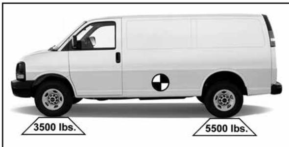
5. If the specific vehicle lift points are not identified, refer to the VEHICLE CENTER OF BALANCE instructions found on our website at
