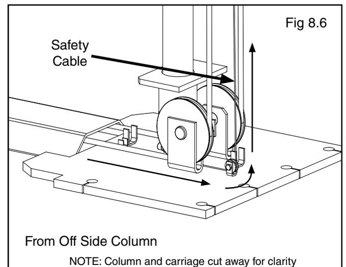
5. Route the cable the same way as on the Power Side going up the Column and over the safety cable sheave.
